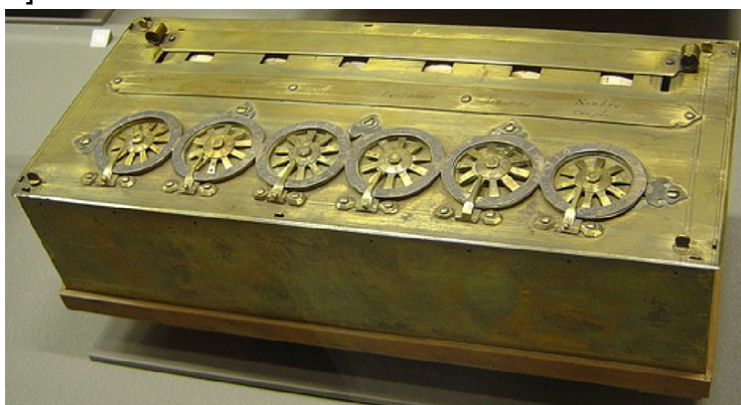
Fig. 1. Pascaline – a calculating machine designed by Blaise Pascal around 1645.
