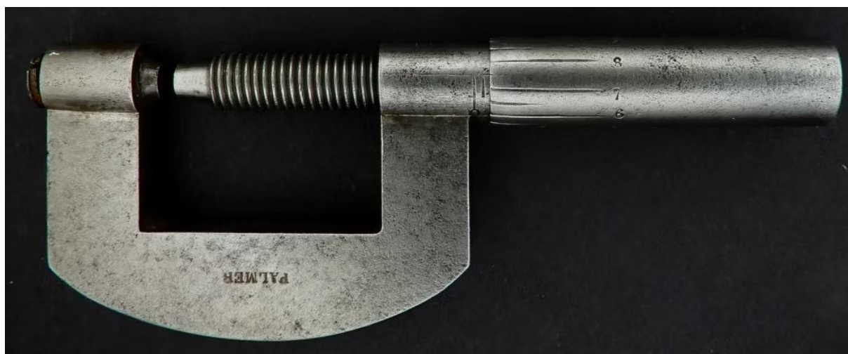
Rys. 21. Mikrometr Jeana Laurenta Palmera ( https://www.robertsonminiatures.com/palmer-micrometer n.d.).
